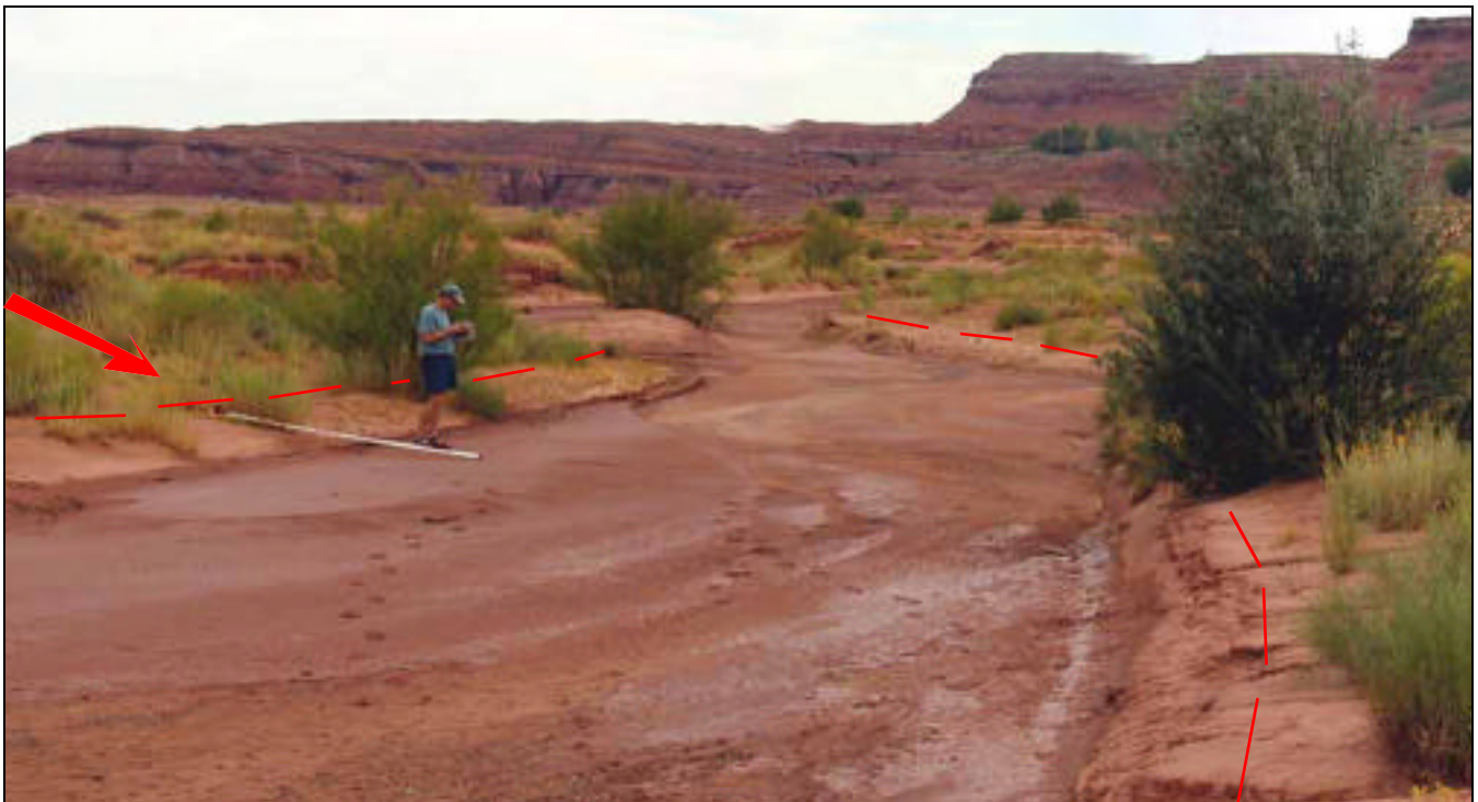
Figure 6. Moenave Wash. Ephemeral, sand bed channels can be very challenging. Bankfull stage lies along the change in slope on the point bar on the far shore. It also corresponds with a vegetation line. It does not match the vegetation on the outside of the meander along the near shore however. Beware of cut-banks especially on the outside of meanders that appear to indicate bankfull stage. They are erosional rather than depositional in nature and not reliable indicators.
